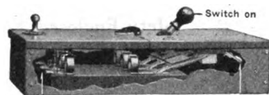
THIS SIDE MUST BE CONNECTED TO LOAD THIS SIDE MUST BE CONNECTED TO LINE CONTACTS CLOSED—COVER CANNOT BE OPENED
